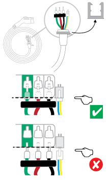
Snap the white levers all the way down on each wire.
