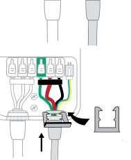
8. Place the wire cover over the exposed wiring. Use a coin to lock the wire cover in place.
