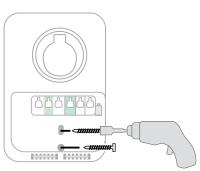
**Note:** If mounting on an exterior wall and bringing power through the rear knockout, apply sealant around the rear knockout to prevent water ingress.
